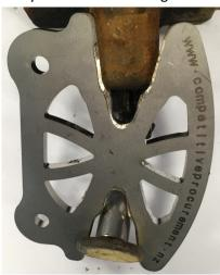
The innermost diameter of the butterfly head fits snuggly around the wire holding the toggle to the twistlock allowing it to be unlocked with little of the metal toggle remaining.
